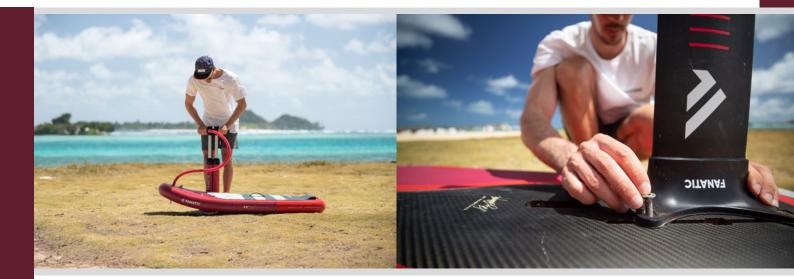
Pump until you reach 15 PSI minimum pressure, for more stiffness you can inflate up to 20 PSI. If it gets too exhausting, switch from double to single stroke action. It's much easier to reach full pressure with single stroke action. Insert the supplied track nuts into the base plate slots. Position your foil on the tracks and align the track nuts under the inserts for the screws. Insert the screws and tighten them.
