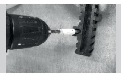
1. Drill the Hole with a 5mm
